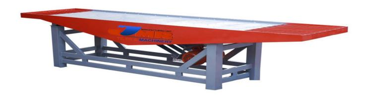
This vibrator has a powerful vibrating unit on its rigid table. It is used mainly to load and foam freshly mixed concrete for U-shaped grooves, boundary blocks, bricks, paver block, interlocking blocks, flyover bricks, blocks, concrete bricks, and etc.
